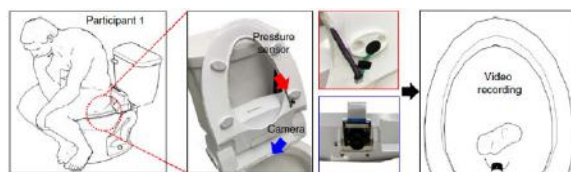
Graphics from Stanford University researchers demonstrating how users were to use the toilet, where the pressure sensor and camera is, and part of what the video camera would record. Photo Credit: Park, Seung-Min, Daeyound D. Won, et. Al. Photo Credit: https://rb.gy/byskdd
