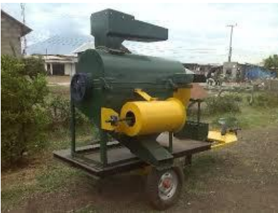
An example of a diesel engine powered maize sheller
